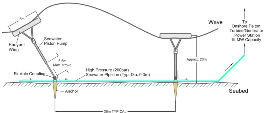
Figure 1: Buoyant wing operation
